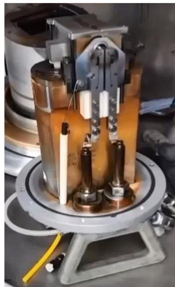
Fig. 1. Ion source following  $\text{AlI}_3$  operation
