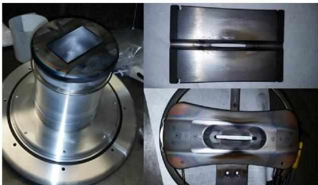
Fig. 2. Ion source following 192 hours of AlI<sub>3</sub> operation with the new bleed system
