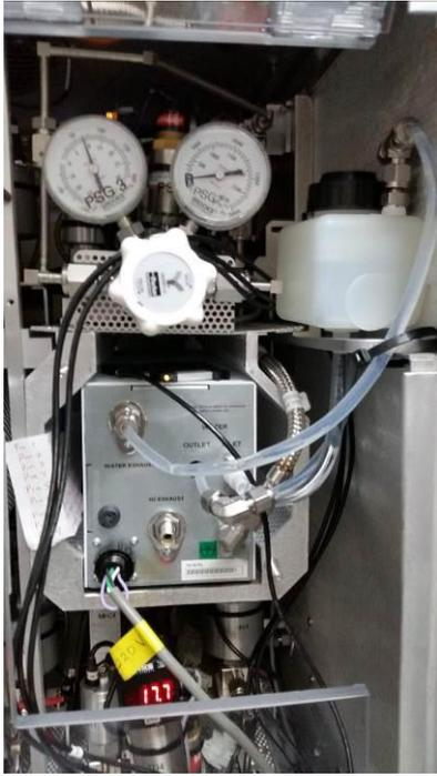
Fig. 4. Hydrogen generator installed in implanter gas box
