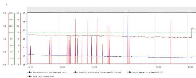
Fig. 3. Stability plot of source running AlI<sub>3</sub> with H<sub>2</sub> feeds into arc chamber and extraction region
