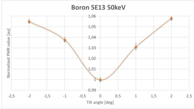
Fig.6. The processed and normalized PMR signal as a function of the implanting tilt angle. The orange curve corresponds to the B implanted samples, while the blue curve is that of the As implanted ones. For color version see the electronic release.
