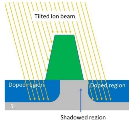
Fig.1. Shadowing effect during ion implantation
