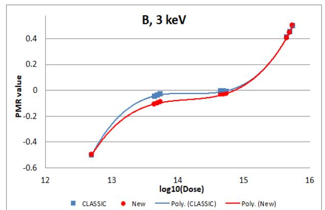
Fig.5. The relativized PMR value as a function of the implant dose. The red curve is measured by the current setup without any insensitive region; while the blue one was obtained before the optical system developments. For color version see the electronic release.
