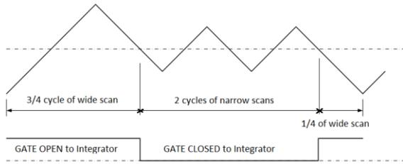
Fig. 4. OptiScan scan waveform with Gate signal.
