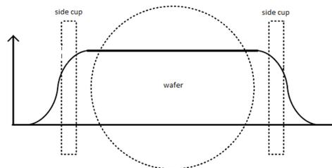
Fig. 3. Side cup current on narrow scans.
