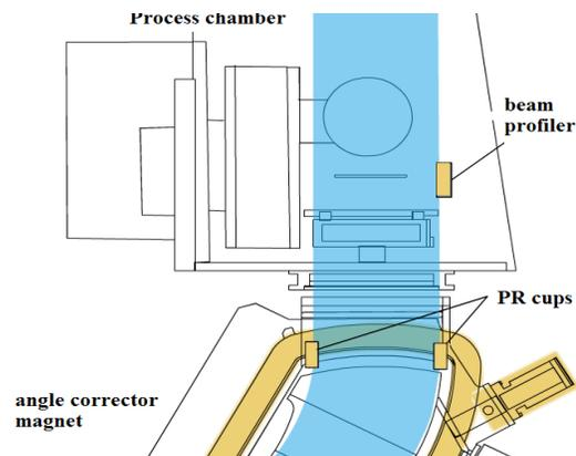
Fig. 1. Placement of PR cups, side cups on Purion XE
