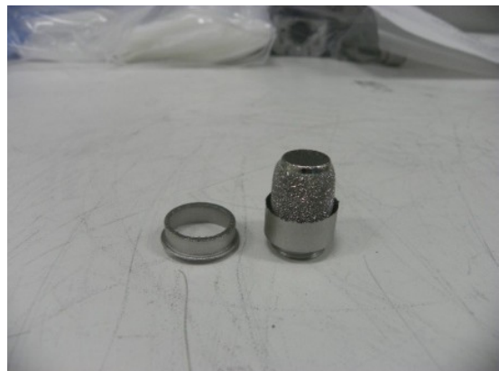
Fig. 4. Photo of a tungsten cathode and its corresponding tungsten cathode shield (tubular member that covers the cathode) after running CO 2 for 20 hours
