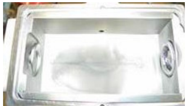
Fig.2. Ion source after 300 hours of GeF 4 and H 2 Co-gas
