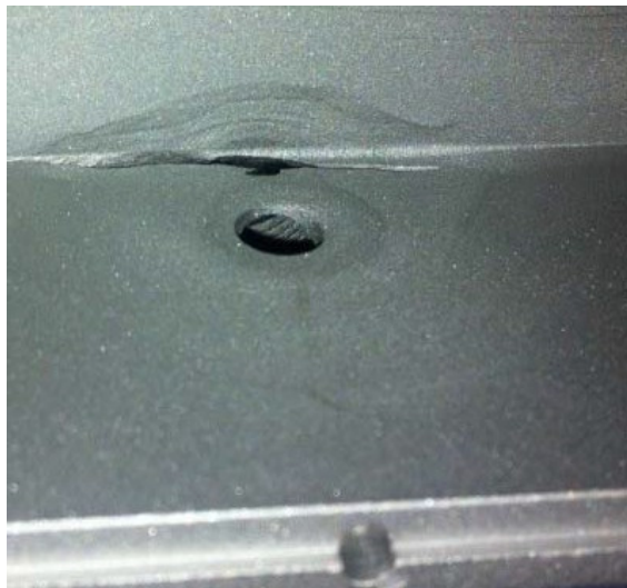
Fig.5. Erosion of the process gas inlet for a W arc chamber body after running dedicated GeF4 for >2000 hours
