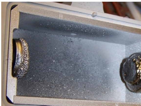
Fig. 1. Halogen cycle/tungsten deposition after 70 hours of GeF 4
